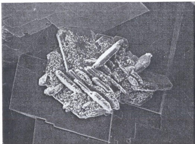
Figure 19. Marcasite—a parallel grouping of tabular plates of dark brown marcasite crystals with an unknown coating. The grouping is 160 micrometers in diameter.
