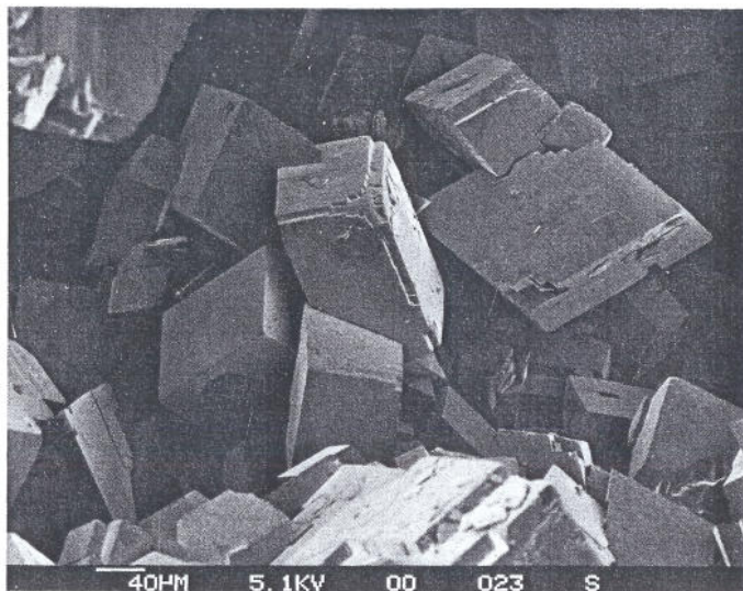
Figure 10. Intergrown rhombohedrons of dolomite. Dolomite, usually white or colorless, is the host mineral upon which all other minerals crystallized. The scale bar is 40 micrometers.
