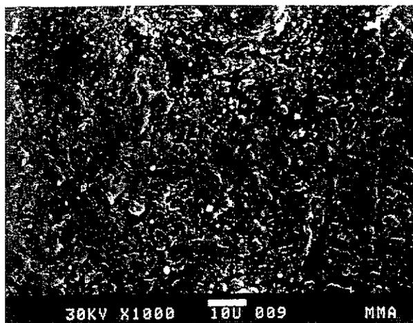
Fig. 2a SEM photomicrograph of Indiana limestone treated with DF-104, in a polished and etched surface. The pre-polymerized resin forms a film as the solvent that covers the calcite grains evaporates.
