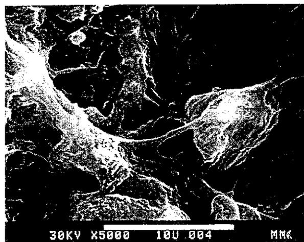
Fig. 1b Detail of the previous photomicrograph showing the resin covering the calcite crystals and the network formed.
