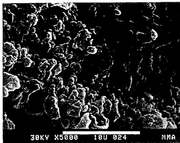
Fig. 3b Detail of the previous photomicrograph showing a detail of a thicker film of resin (top right corner) which fades into a thinner film (lower right-hand side) characteristic of the appearance of this treatment, and a non-impregnated part of Indiana limestone (bottom left corner).
