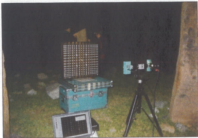
Figure 10. System calibration (foreground) and cleaning monoliths (behind calibration plate) with bamboo skewers and toothbrushes to remove accretions
