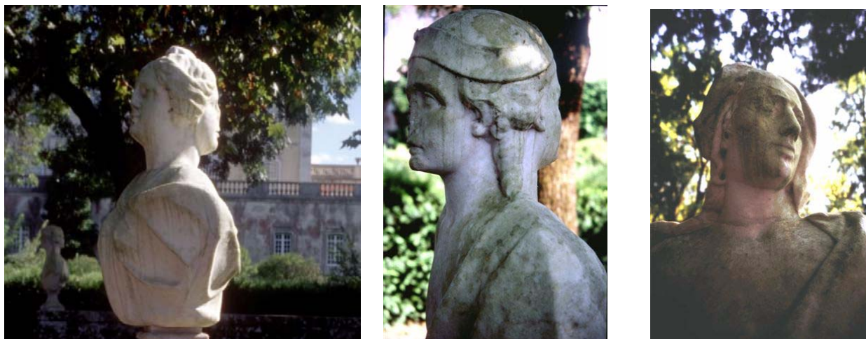
Figure 4: Three bi-face busts to which an aqueous emulsion of an oligomeric siloxane was applied after cleaning in 1999, four years before the photograph was taken (Photos 2003). Note the difference in biocolonization depending on the location of the busts. From left to right, increasing shade.
