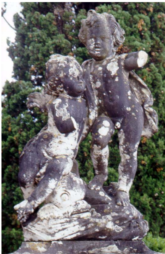
Figure 1: Appearance of a putti group before the intervention in 1996/7. Note the dark soiling resulting from biocolonization. This same group is shown in Figure 3 some years after cleaning.
