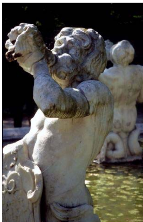
Figure 2: The streaking pattern is particularly noticeable under the arm of the Triton. The pattern results from uneven biocolonization. The marble statues are in a fountain that had been cleaned and treated with a water repellent four years before the photograph was taken (Photo 2003).
