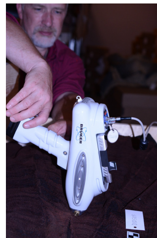
Kevin P. Smith, Haffenreffer Museum of Anthropology using a pXRF on a 14th century gown from Herjolfsnes, Greenland at the National Museum of Denmark. (Photo MHS)
