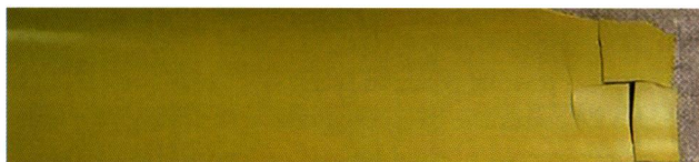
Fig. 3 (a, b, c). Figure 3a shows the drying of a lead tin yellow in cold pressed linseed oil. Figure 3b shows the mechanical properties of lead-tin yellow in cold pressed linseed oil at different aging stages. The figure also shows the effects of changing relative humidity in the mechanical behaviour of the sample tested. Figure 3c shows a picture of a lead-tin yellow in cold pressed linseed oil paint film only after 18 years of ageing at room conditions
