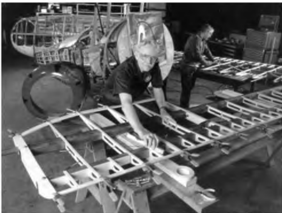
Max Gainer, left, restoration volunteer at the Paul E. Garber Facility, and Rich Horgan, restoration specialist, work on the wings of the Nieuport 28C.1. (Photo by Carolyn Russo)
