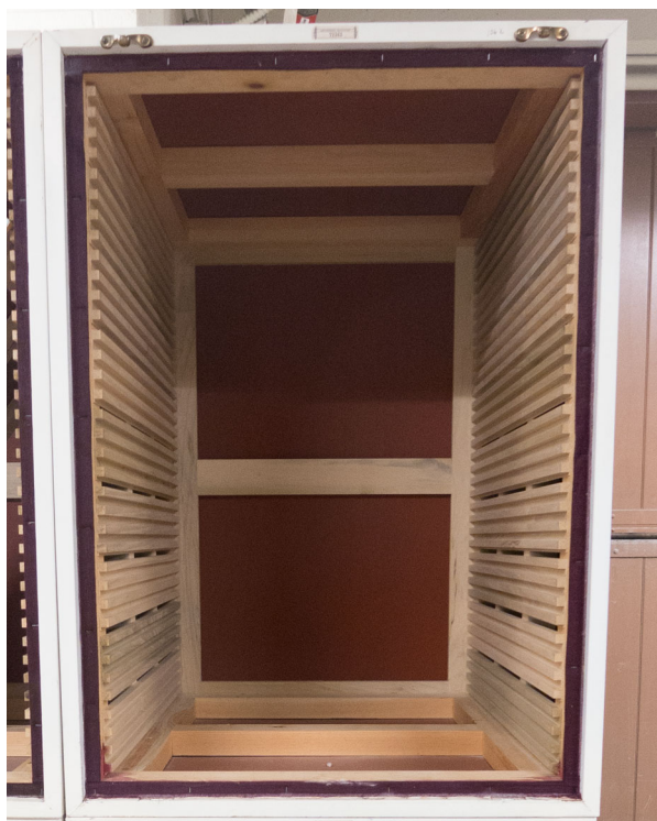
FIG. 1. Example of an empty wooden storage cabinet. Note that the cabinet is accessed by removing the door, and both are constructed of a wood frame with metal cladding. Wooden drawers (not pictured) can be installed, as needed, in the wooden tracks. The gasket material is red felt.
