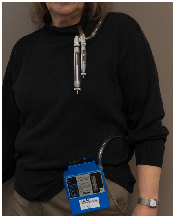
FIG. 4. Detail of an employee wearing a personal exposure sampler, consisting of a pump clipped onto the pants' waistband and the sampling media clipped to the collar, to monitor the air within the employee's "breathing zone."
