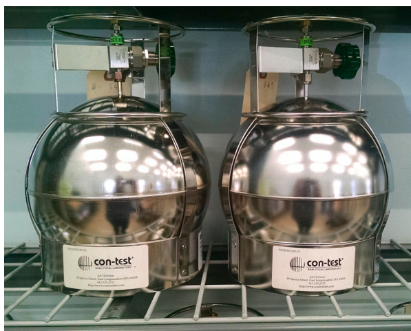
FIG. 3. Image of two SUMMA® canisters, similar to those used in this study to carry out testing according to “Compendium Method TO-15 for Determination of Volatile Organic Compounds (VOCs) in Air Collected In Specially-Prepared Canisters and Analyzed by Gas Chromatography/ Mass Spectrometry (GC/MS)”. Image credit: Con-Test, 2017.
