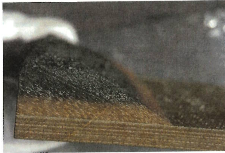
Fig. 5.2 Mercury 7, 1962, cross-section through the ablated upper part of the heat shield, illustrates layers of the fiberglass cloth laminate saturated with phenolic resin (NASM 1968-0263-002; image 2008 H. Szczepanowska)
