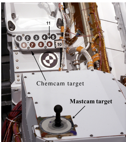
Fig. 1. Portion of Mastcam image acquired during pre-flight rover testing showing Mastcam and ChemCam calibration target (CCCT) locations on rover deck. CCCT targets numbered, including target holder (Target #11) used for calibration of passive spectra.
