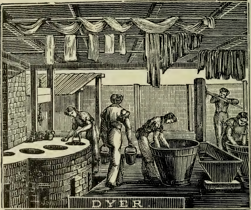
FIGURE 2.—The earliest known illustration of the interior of an American dye house (Hazen, 1836). Left: A worker lifting a dye bucket from a vat heated by a furnace that encases the vat. Right: Workers bent over various vats. The cloths draped on overhead beams indicate that finished cloth was being piece-dyed here.
