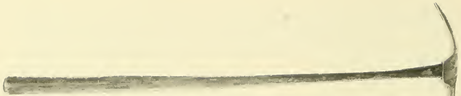
Figure 45.—19TH CENTURY: THE UPHOLSTERER'S HAMMER is an unknown; it is not dated, its maker is anonymous, as is its user. It is of American origin, yet of a style that might have been used in England or on the Continent. This lack of provenance need not detract from its significance as a material survival. This hammer, the brace (fig. 46), the bevel (fig. 47), and the compass saw (fig. 48) are sufficiently provocative in their design to conjure some image of a technology dependent upon the skilled hand of craftsmen working in wood and of the relationship between the hand, the tool, and the finished product. (Smithsonian photo 49793-A.)
