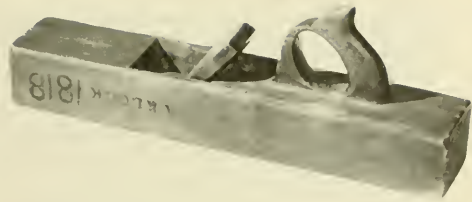
Figure 26.—1818: THE JACK PLANE, used first by the carpenter for rapid surfacing, is distinguished primarily by the beveled and slightly convex edge of its cutting iron. As with the plow and the rabbit, its shape is ubiquitous. Dated and marked A. Klock, this American example follows precisely those detailed in Sheffield pattern books. (Smithsonian photo 49794-C.)
