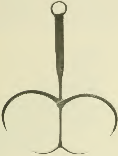
Figure 20.—EARLY 19TH CENTURY: THE DOUBLE CALIPERS of the woodturner permitted double readings to be taken without changing the set of the tool. Inherent in this practical design is a gracefulness of line seldom surpassed. (Private collection. Smithsonian photo 49793-C.)
