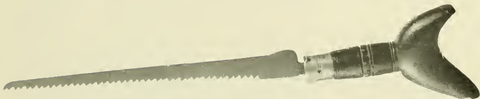
Figure 48.—18TH CENTURY: THE HANDLE OF THE COMPASS SAW, characteristically Dutch in shape, is an outstanding example of a recurring functional design, one which varied according to the hand of the sawer. (Smithsonian photo 49789-C.)
