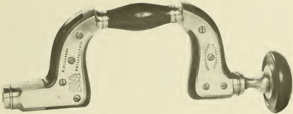
Figure 57.—1876: JAPANED AND SPLINTED WITH HEAVY BRASS, this brace was among the award-winning tools exhibited at the Centennial by E. Mills and Company of Philadelphia. (Smithsonian photo 49792 D.)
