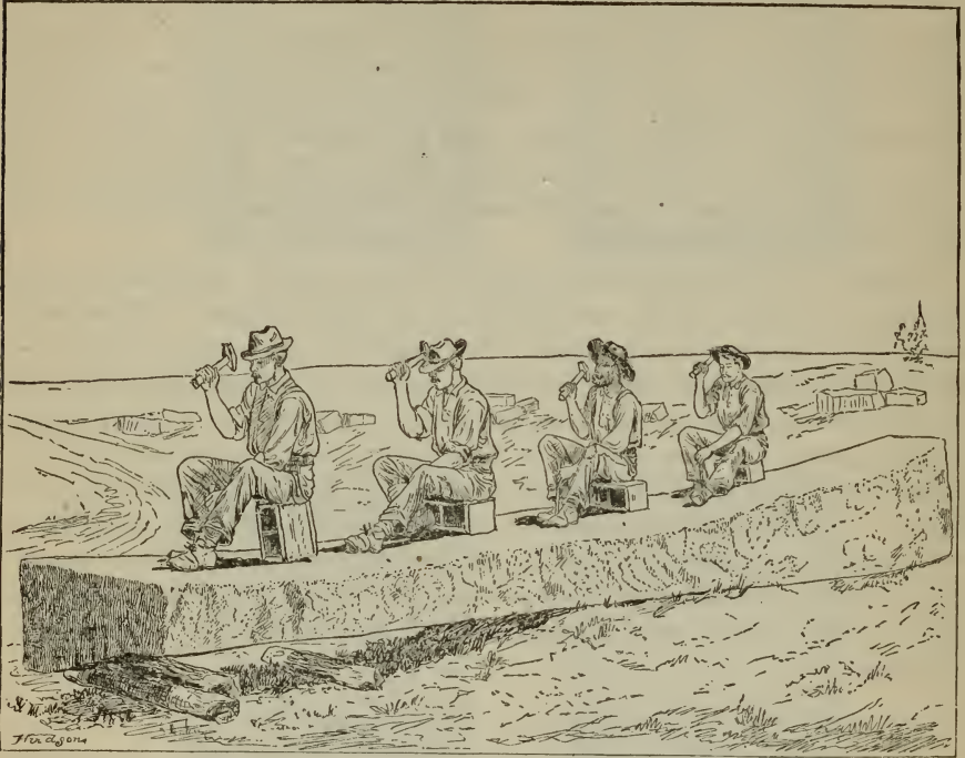
Drilling holes for splitting stone with plug and feathers.
