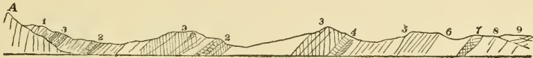
FIG. 131.—Section of Taconic Rocks. A, Primary schists; 1, granular quartz, or brown and white sandstone; 2, 2, Stockbridge limestone; 3, 3, magnesian slate; 4, Sparry limestone; 5, Taconic slate; 6, roofing slate; 7, rough coarse siliceous beds; 8, flinty slate; 9, Hudson River shales. (After E. Emmons.)
