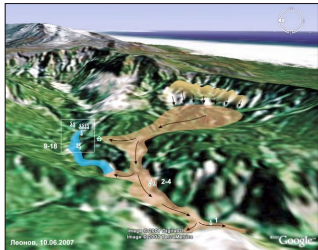
Figure 18. An oblique aerial view created on a base map from Google Earth software, depicting the Valley of Geysers looking E (N is to the left). The slide area and direction of flow are clearly marked, the mass having swept down the caldera's E wall. The topographically flat area in the upper right is the Pacific ocean. Note lodge at small icon in the form of a house. Thermal features indicated by symbol for spring (small circles with tail); many of these are numbered. The image also shows where the slide dammed the Geyzernaya river; the resulting lake submerged the Bolshoi and Maly geysers. Courtesy of Vladimir and Andrei Leonov.
