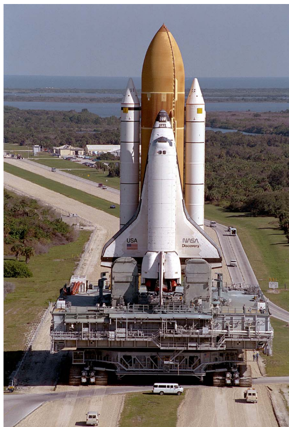
Fig. 19. The same approach as used for the Saturn V launch process has been followed by the Space Shuttle program. Here the Space Shuttle rides on the crawler transporter en route to Launch Complex 39. Note the vehicles shown for the scale of this vehicle. (NASA photograph.)
