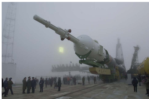
Fig. 22. From the earliest times of the Soviet Union’s space program it decided to move launchers horizontally by rail from the assembly building to the launch complex. Presently at Baikonur Cosmodrome, the principal Russian spaceport, payloads to be fired into orbit are prepared for launch in a processing center a few kilometers from the launch site. The overall testing as well as fueling and pneumatic pressurization of the spacecraft take place there, and then the payloads are integrated with the rocket’s upper stage. All of the rocket stages are sent by rail from the production plant, and mated for launch at this assembly point, before being loaded by cranes on a flat railroad transporter that will take it to the launch site, raise it vertically, and fire it into space. Here the Russian TM-31 Soyuz spacecraft approaches the launch complex on the horizontal rail car in preparation for its launch with a crew of three on October 31, 2000. (NASA photograph.)
