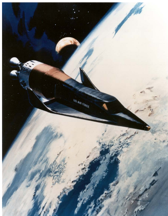
Fig. 28. The United States also pursued the X-20 Dyna-Soar in the 1960s, a military spaceplane to be launched atop a newly developed launcher. The U.S. Air Force believed that the X-20 would provide long-range bombardment and reconnaissance capability by flying at the edge of space and skipping off the Earth’s atmosphere to reach targets anywhere in the world. Begun on December 11, 1961, this spaceplane was always troubled by the absence of a clearly defined military mission. Accordingly, in 1963, Defense Secretary Robert S. McNamara canceled the program. (DoD illustration.)
