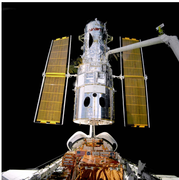
Fig. 13. Attached to the “robot arm” the Hubble Space Telescope is unberthed and lifted up into the sunlight during the second Space Shuttle servicing mission designated HST SM-02 in 1997. (NASA photograph.)
