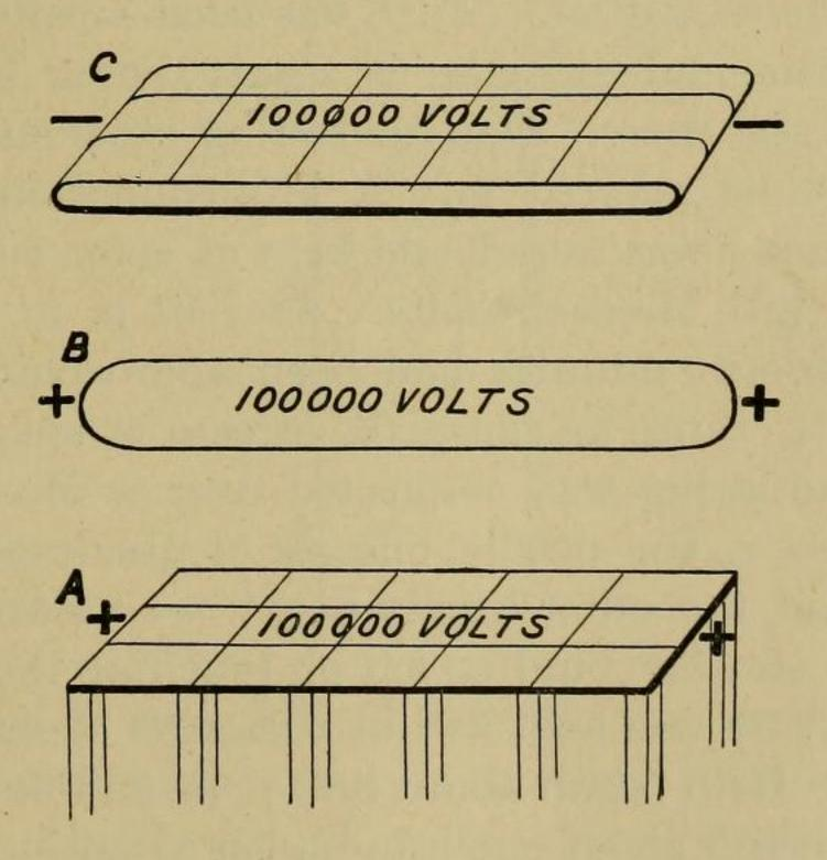
of low potential. Thus in the accompanying diagram if A represents a highly charged (and by this we mean voltages in the hundred thousands) insulated conductor, B a mobile conductor charged equally high and same sign as A, then C an oppositely charged mass, B will move from A to C.
