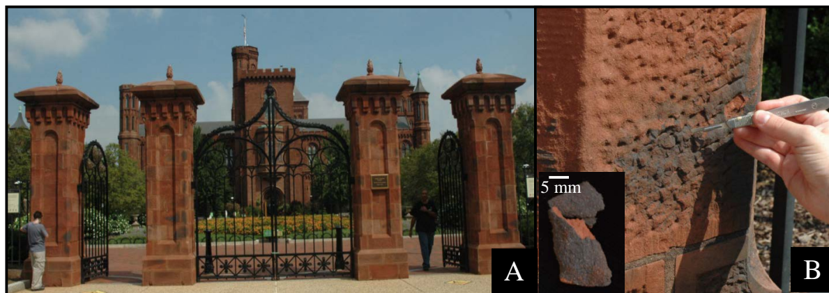
Figure 1 A) Gated entrance to Haupt Garden with Smithsonian Castle in background. B) Sampling black-stained areas on gatepost. Inset: fractured fragment taken from gatepost.
