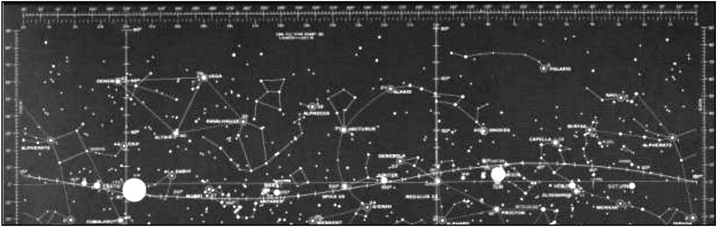
Apollo 11 star charts. This was prepared especially for the position of the stars, Earth, Sun, and Moon at the time of the Apollo 11 launch, July 1969. Slightly different charts were prepared for Apollo VIII and would have been carried onboard. Note the two-digit numbers for many of the stars—these numbers were keyed in as a “noun” into the Apollo Guidance Computer’s DSKY. Credit: NASA
