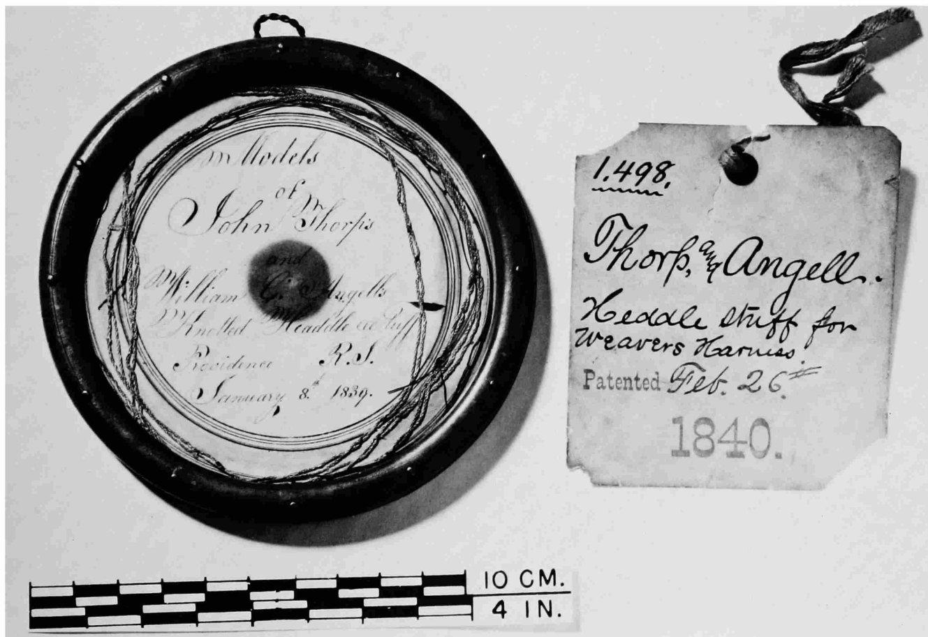
FIGURE 74.—Framed individual heddles, patent model 1498. (S.I. neg. 80-12385)
