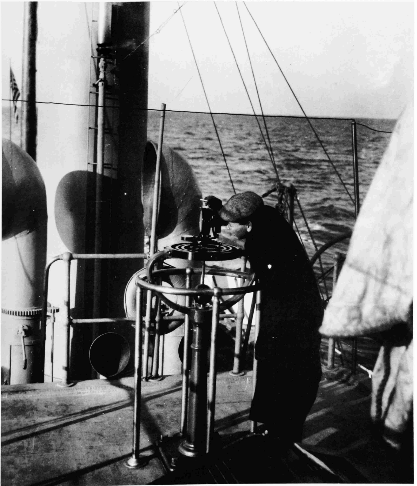
FIGURE 66.—Magnetic observations at sea, aboard the ship Bache off Puerto Rico, 1904. The dip circle in use is similar to the Lloyd-Creak instrument in the present collection (No. 37, Figure 65).
