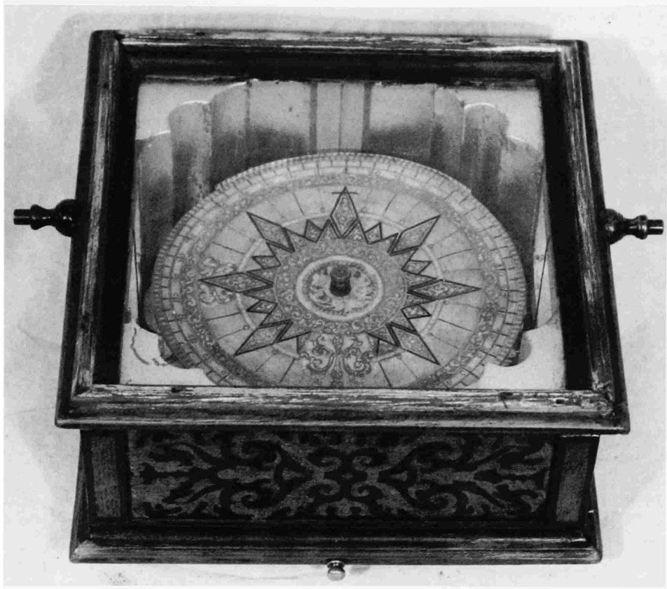
FIGURE 1.—Navigational compass, 15th century, Portuguese, a typical instrument in which a magnetized needle is fixed to the underside of a circular card on which the directions are laid out. (Copy, in the Smithsonian Institution, of an original in the Museum of the History of Science, Cambridge University.)
