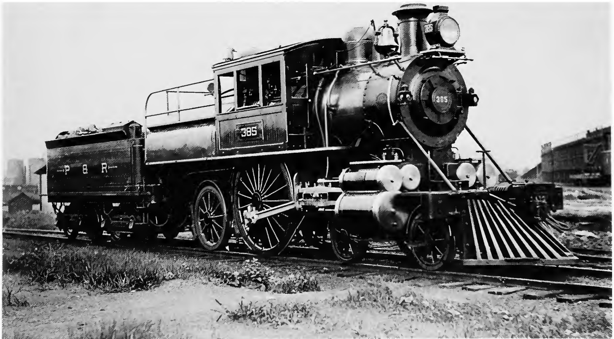
FIGURE 9. America's final effort to test the single for express service is represented by the Philadelphia and Reading's 385. She was produced by Baldwin in 1895. (Photograph courtesy of Thomas Norrell.)
