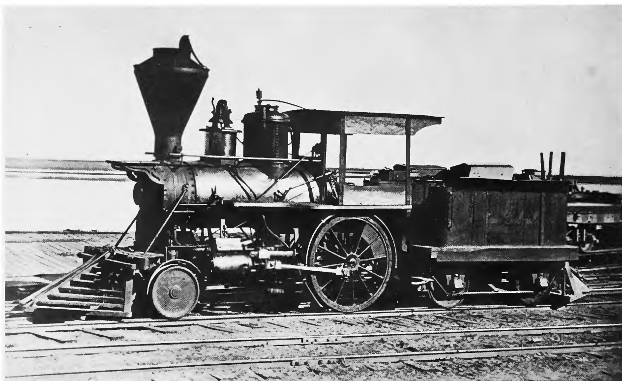
FIGURE 15. Several singles saw service on the West Coast, and a few were even constructed in that region. The San Gabriel was built in 1864 by the Vulcan Iron Works of San Francisco, reportedly for the San Francisco & Alameda Railroad. (Photograph courtesy of the Los Angeles County Museum of Science.)
