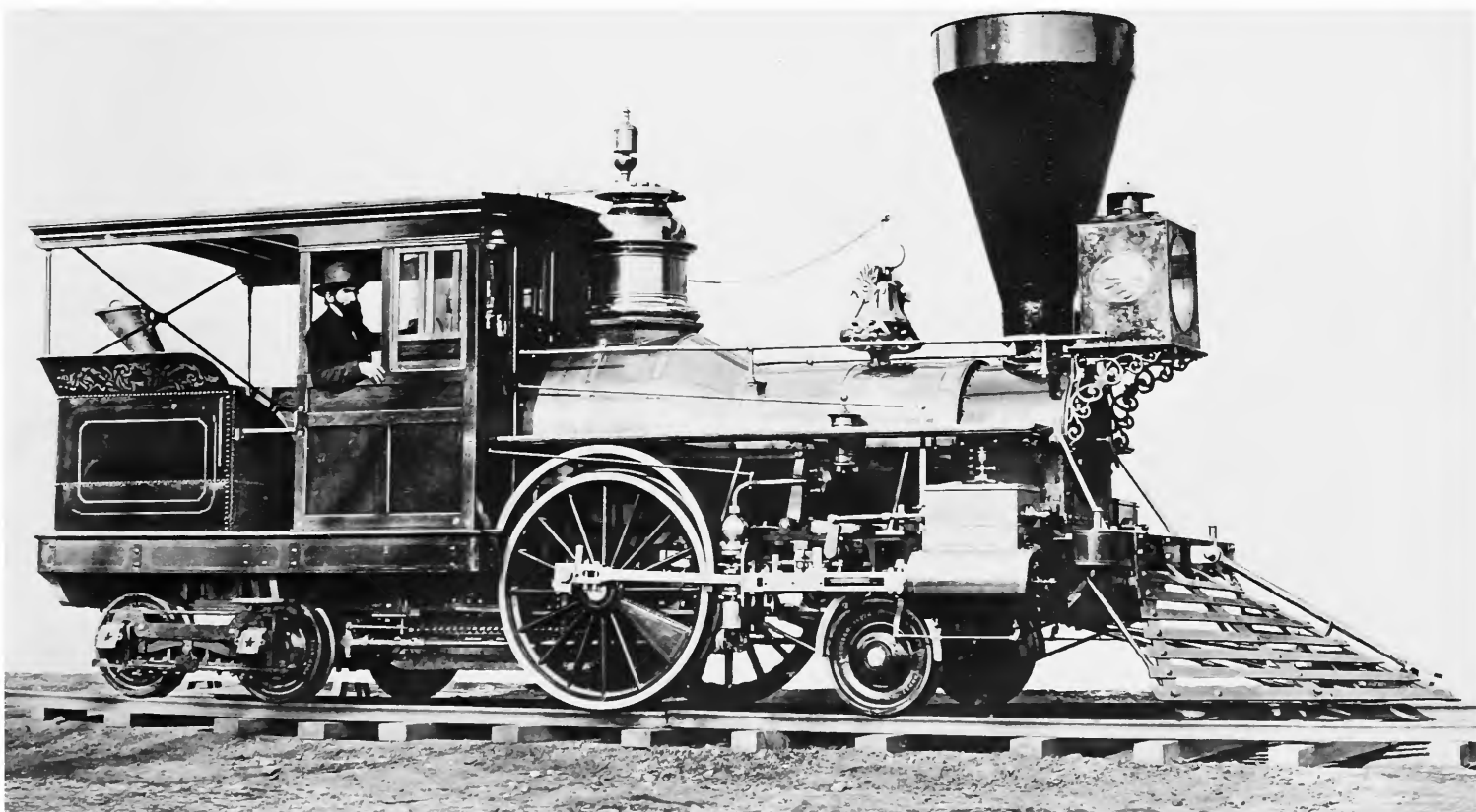
FIGURE 13. Danforth, Cooke & Company produced a number of single-driven tank engines for suburban and branch-line service in the 1850s and 1860s. The engine shown here is thought to be the Central Railroad of New Jersey's Wren or Pewit of 1864. (Photograph courtesy of Thomas Norrell.)
