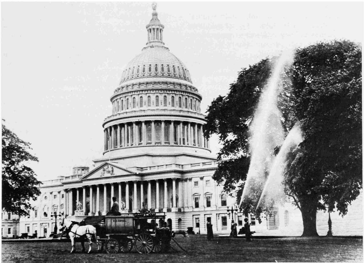
FIGURE 31.—Fitzhenry-Guption power sprayer (1908), seen here spraying for elm leaf beetles on the grounds of the U.S. Capitol, May 1911. (Catalog No. 366.)
