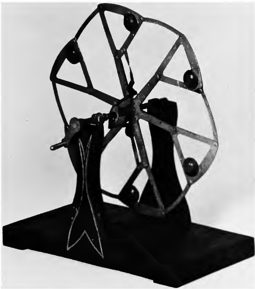
FIGURE 17.—Patent model of H. N. Throop's governor for marine steam engines, 1857. (NMHT 325612. Smithsonian photo 69388.)
