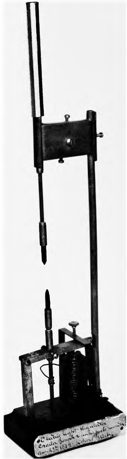
FIGURE 130.—Patent model of arc lamp by Charles J. Van Depoele, 1880. (NMHT 252652. Smithsonian photo 71877.)
