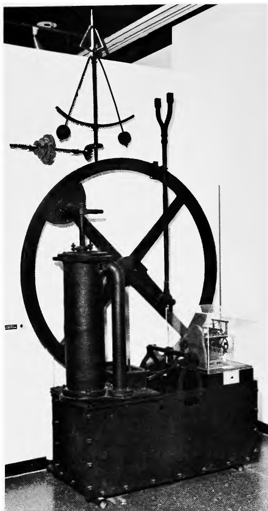
FIGURE 4.—Steam engine built in 1819 by John Holloway of Philadelphia. In the arrangement shown, the governor is not connected to the engine. Originally it was installed on the floor above the engine. (NMHT 319405. Smithsonian photo 72169.)
