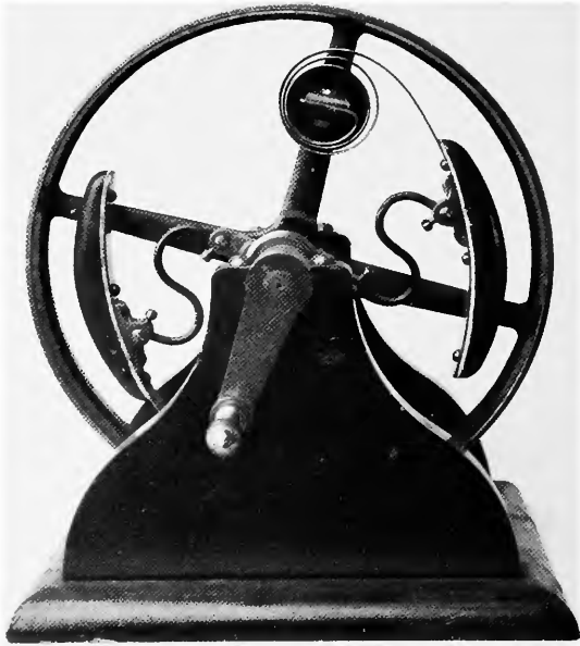
FIGURE 37.—Patent model of shaft governor by Daniel A. Woodbury, 1870. (NMHT 251290. Smithsonian photo 30362.)
