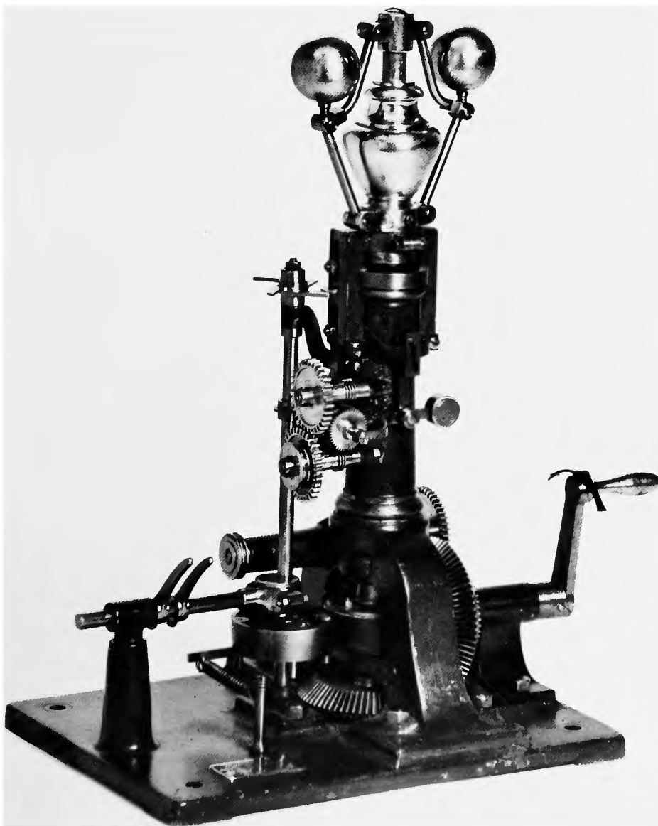
FIGURE 26.—Patent model of engine governor by Johann Georg Bodemer, 1876. (NMHT 309243. Smithsonian photo 69389.)
