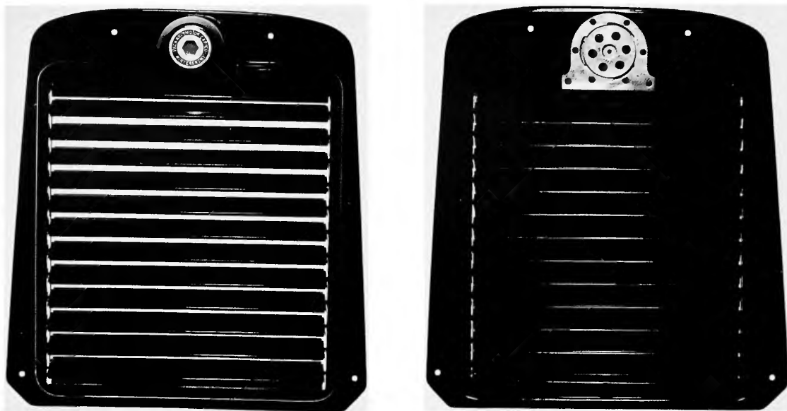
FIGURE 103.—Packard “Winterfront,” 1920s: view from front and back. The shutters are operated by a thermostat (top center) which senses the radiator temperature through metal contact. (NMHT 329286. Smithsonian photos 71537, back, and 71538, front.)
