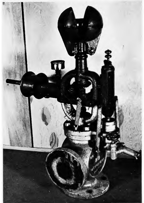
FIGURE 36.—Governor for steam-driven air compressor built by the Jarecki Mfg. Co., about 1920. (NMHT 326536. Photo CLG.)
