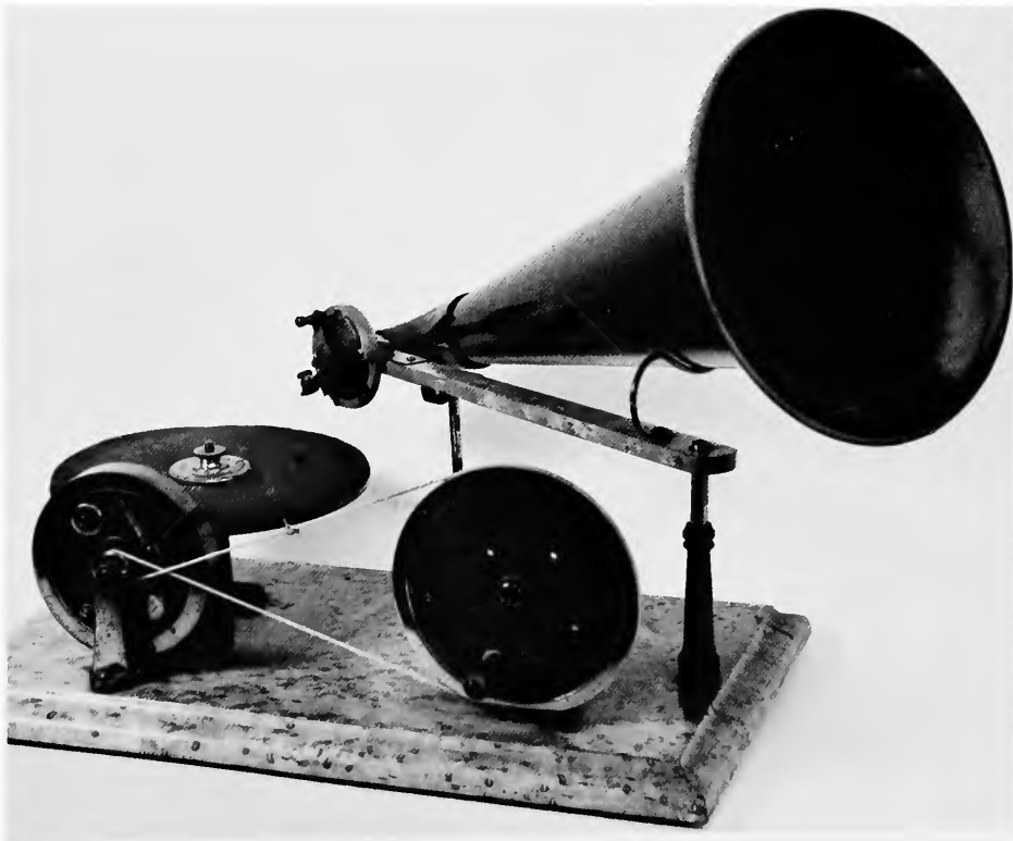
FIGURE 75.—Berliner gramophone equipped with governor (left) invented by Alfred C. Clark, 1898. (NMHT 253757. Smithsonian photo 42171-E.)
