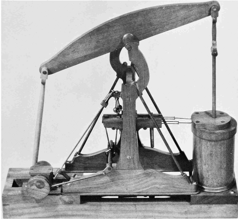
FIGURE 7.—George H. Corliss's patent model of 1849 describing his basic patent of automatic cutoff control. (NMHT 308646. Smithsonian photo 31694.)
