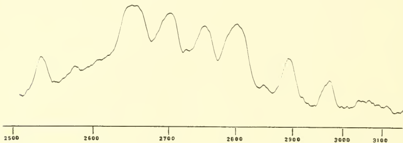
FIG. 4.—Photometric record of algal spectrogram of mercury arc.
