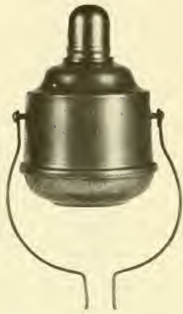
Figure 51.—NICKEL TORCH with nipple over the burner, 1888. (Smithsonian photo 49926-E.)
