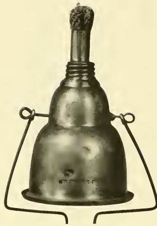
Figure 52.—BRASS TORCH FOR CAP, 1888. (Smithsonian photo 49927-B.)
