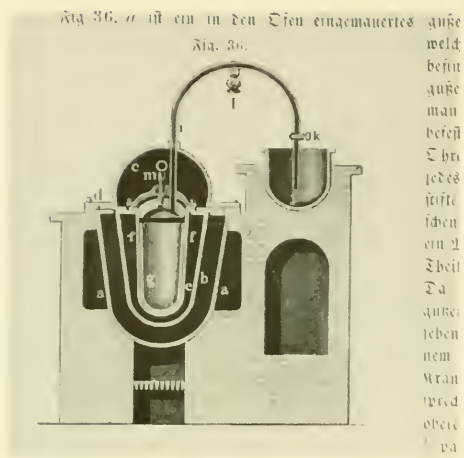
Figure 4.—APPARATUS FOR CONVERTING WHITE PHOSPHORUS into the red allotropic form, 1851. Redistilled phosphorus is heated in the glass or porcelain vessel (g) which is surrounded by a sandbath (e) and a metal bath (b). Vessel (j) is filled with mercury and water; together with valve (k), it serves as a safety device. The alcohol lamp (l) keeps the tube warm against clogging by solidified vapors. Because of hydrogen phosphides, the operation, carried out at 260° C., had to be watched very carefully. (According to Arthur Albright, 1853; reproduced from HUGO FLECK, Die Fabrikation chemischer Produkte . . . , page 112.)
