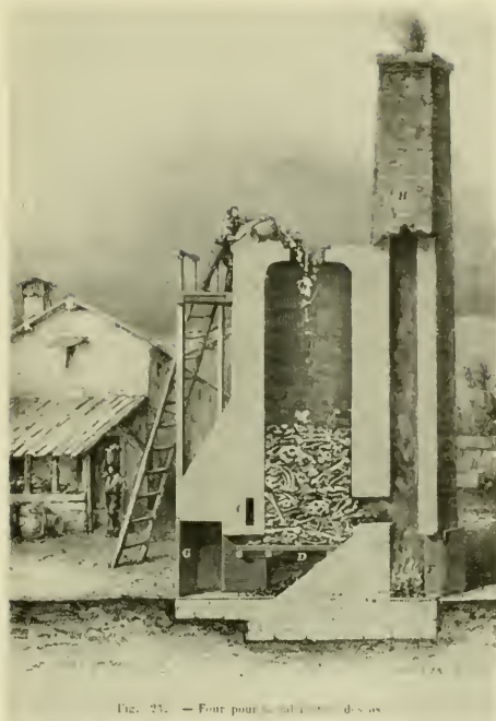
Fig. 25. — Four point calcination of bones.
