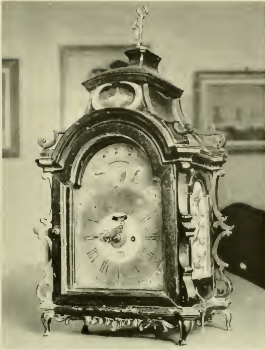
Figure 29. —TABLE CLOCK BY BERTOLLA in the collection of Doctor Vittorio dal Lago of Bergamo. The dial indicates the days of the week and of the month, the names of the months and lunar phases. The clock strikes the hours and quarters and repeats. (Courtesy of Sig. Luigi Pippa of Milan.)
