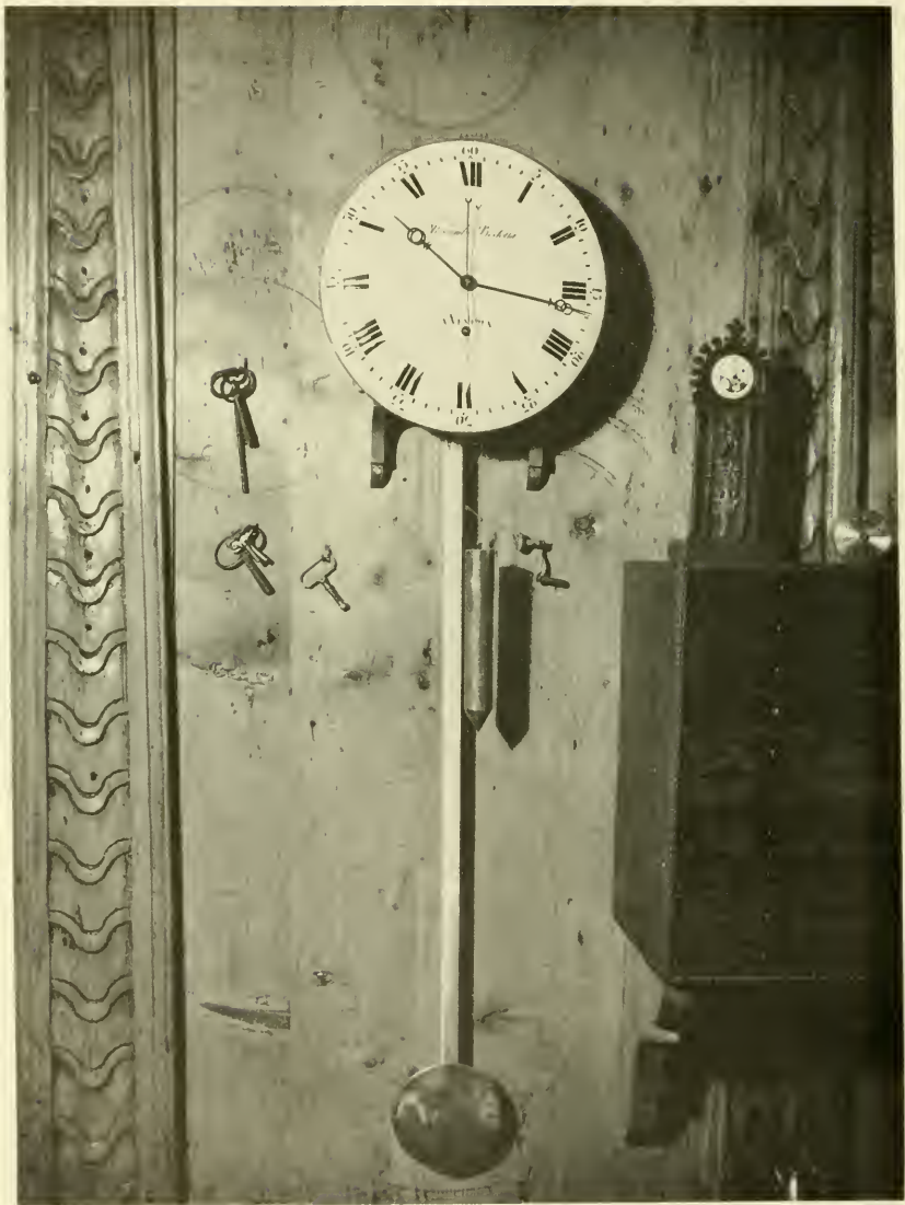
Figure 28.—DETAIL OF WALL of Bertolla's workshop, with regulatory clock made by his nephew, Alessandro Bertolla of Venice. Note wheel layouts, etc., scribed in the paneling. (Courtesy of Museo Nazionale della Scienza e della Tecnica, Milan.)
