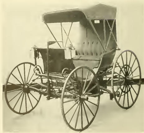
FIGURE 1.—DURYEA AUTOMOBILE in the Museum of History and Technology, from an 1897 photograph. The gear-sprockets were already missing when this was taken, and the chain lies loosely on the pinion. Shown at the right, the Duryea vehicle following the recent restoration (Smithsonian photo 34183).
