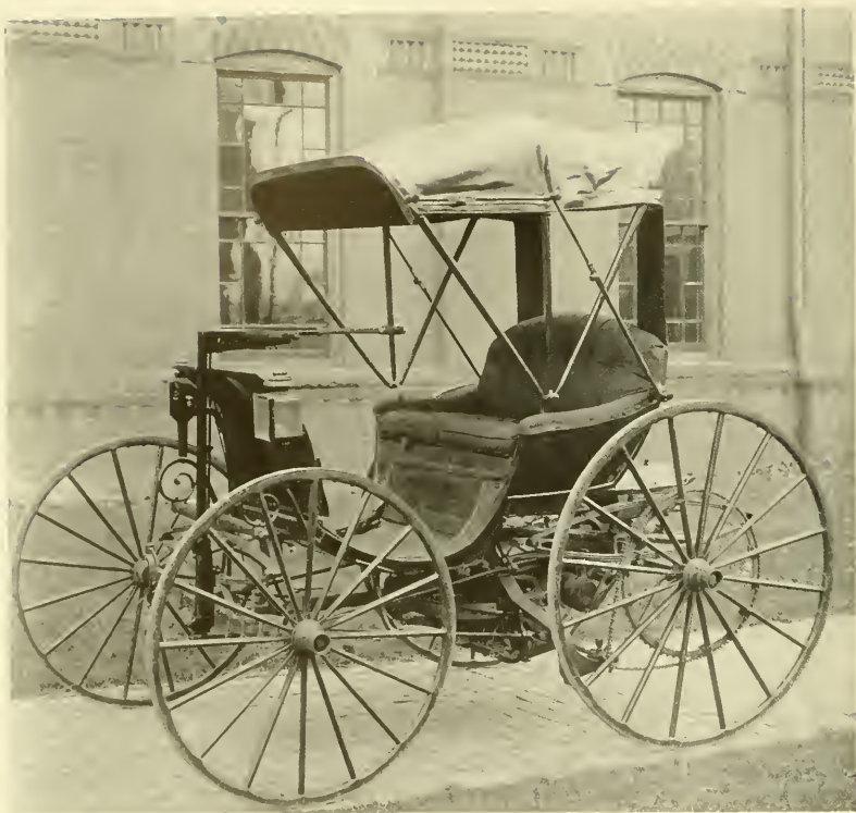
FIGURE 1.—DURYEA AUTOMOBILE in the Museum of History and Technology, from an 1897 photograph. The gear-sprockets were already missing when this was taken, and the chain lies loosely on the pinion. Shown at the right, the Duryea vehicle following the recent restoration (Smithsonian photo 34183).
