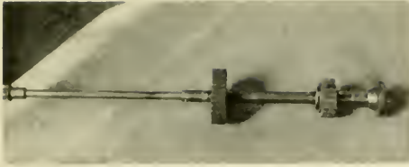
FIGURE 25.—HALF OF JACKSHAFT, showing rawhide gears, double shrouded pinion and half of the Columbia differential.
