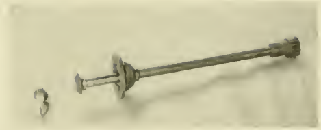
FIGURE 26.—HALF OF JACKSHAFT showing double-shrouded pinion and half of the Columbia differential.
