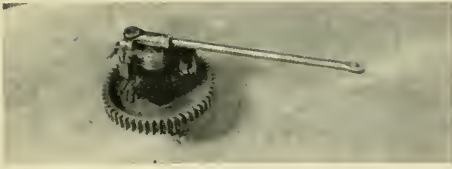
FIGURE 19.—UNDER SIDE of exhaust valve mechanism showing electrical contacts that give spark only on every other revolution.
