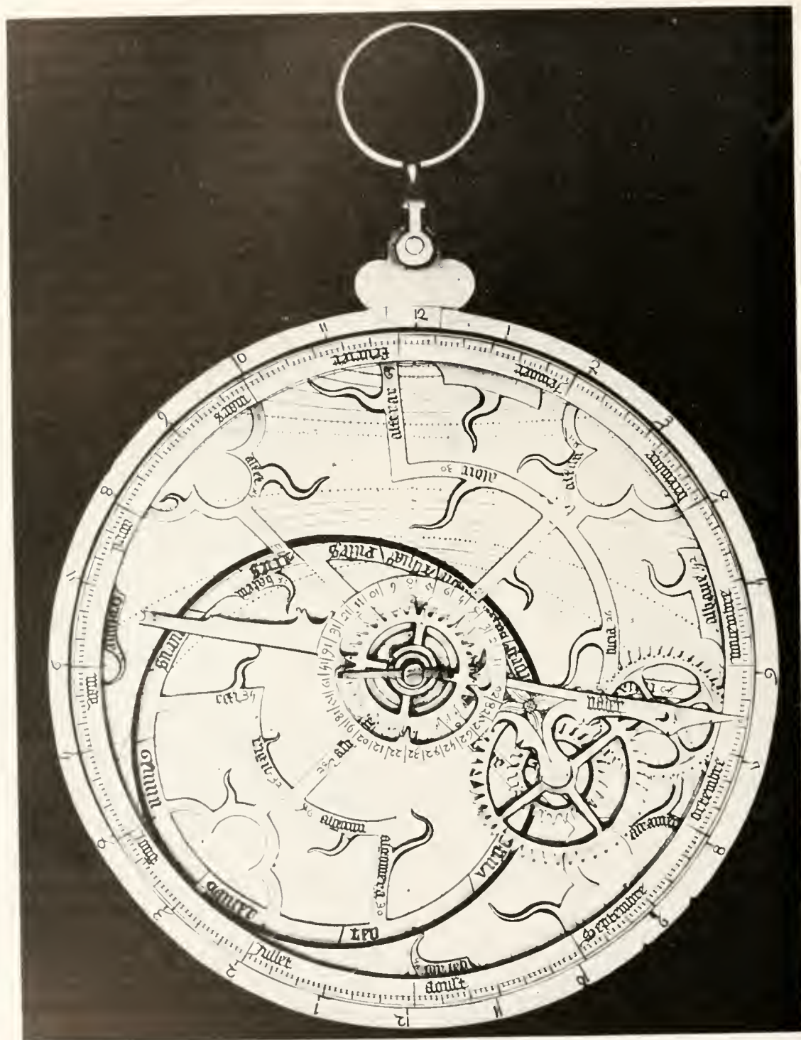
Figure 17. FRENCH GEARED ASTROLABE OF TREFOIL GOTHIC DESIGN, ca. A. D. 1300. The gearing on the pointer is, from the center: (32)/14-45+27-39 , the last meshing with a concave annular gear of 180 teeth around the rim of the rete of the astrolabe. A second pointer, geared to this so as to follow the Moon, seems to be lacking. (Photo courtesy of Science Museum, London.)
