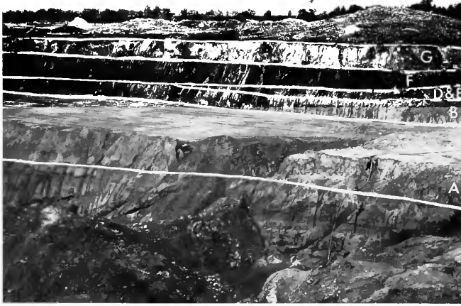
FIGURE 8.—West wall of the pit showing the thinning of unit F to the north-northeast (channeled out by river system?). To the left of center in the photograph, the channel cuts down to unit B; units D and E have been completely removed. Below the working ledge of the pit are the fine, clayey sands of the Yorktown Formation.
