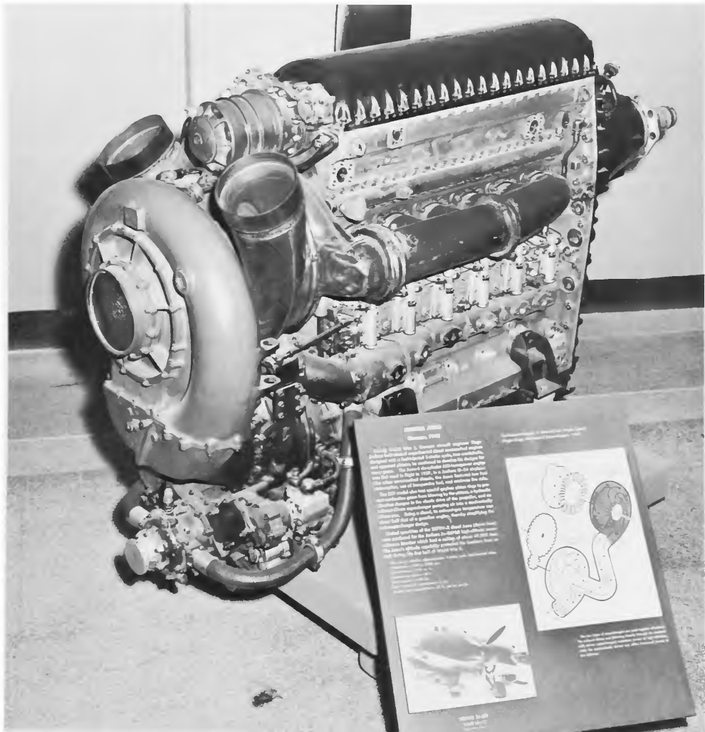
Figure 60.—Junkers Jumo 207-D 2-stroke-cycle 6-cylinder opposed-piston diesel engine (NASM 1966-13); 1200 hp at 3000 rpm, 1430 lb. Photograph shows engine equipped with exhaust-driven turbo-supercharger as used in high-altitude German reconnaissance airplane in World War II. Earlier unsupercharged versions (rated 750 hp at 1800 rpm, 1650 lb) were used in pre-war commercial airplanes. (Photo A-3112)
