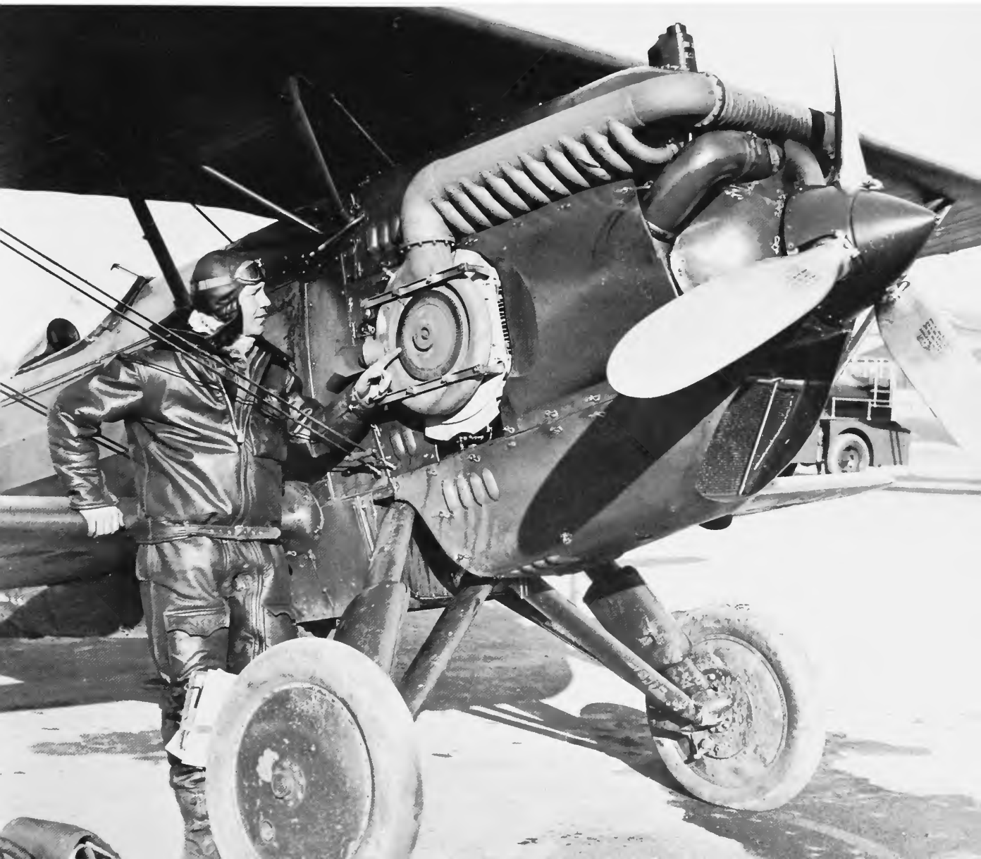
Figure 66.—Side-type turbo-supercharger installed on Curtiss D-12F 460-hp engine in Curtiss P-5 Hawk, 1927. This exposed position of the turbine wheel was effective in reducing the blade temperature as compared to the earlier arrangement shown in figure 65. (Photos A-3094)
