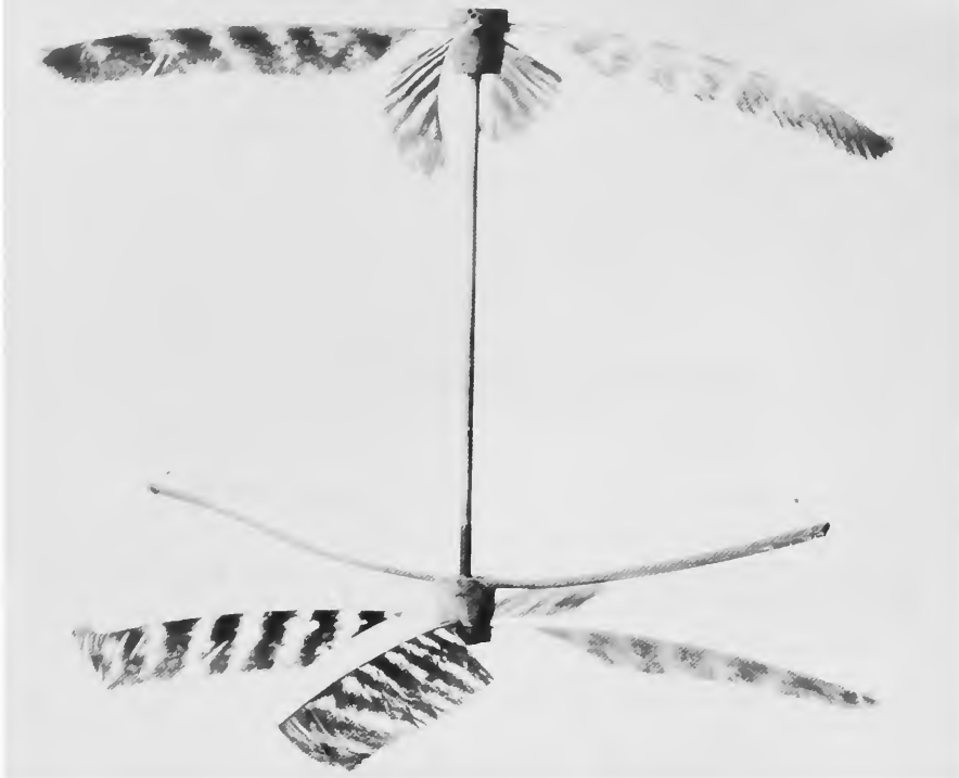
Figure 1.—Reproduction of Launoy and Bienvenue helicopter (NASM 1930-15), using bent-bow propulsion, 1784. (Photo A-18232)
