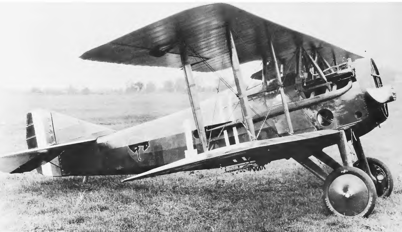
Figure 30.—An Hispano-Suiza V-8 powered this Spad 7 airplane, used by 27th Squadron, AEF, World War I, 1917–1918, (Photo A-44832-C)
