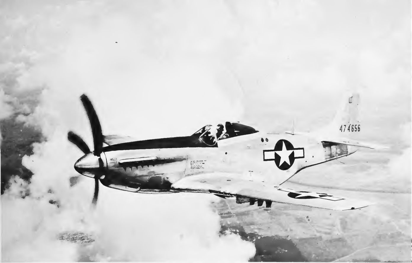
Figure 56.—Liquid-cooled fighter, North American P-51 Mustang of World War II. Coolant radiator is housed under fuselage, below the star insignia. Inlet and outlet ducts are designed to minimize drag. (Photo A-45801)
