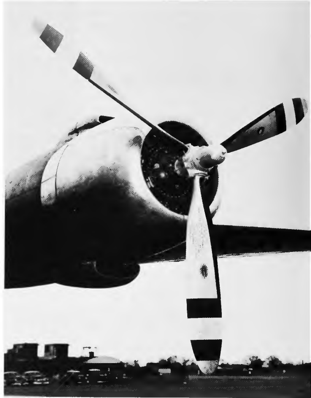
Figure 54.—Installation of radial engine on a Douglas DC-6, 1949, showing modern cowling for radial engine, with controllable outlet flaps. (Photo A-50822)
