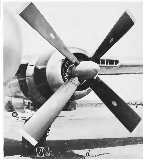
Figure 68.—Propeller development: a , Langley wood propeller (NASM 1938-56E) of 1893, used on Aerodrome No. 4. b , Curtiss-Reed twisted-duraluminum propeller (D-6), 1925. c , Hamilton-Standard 2B20 constant-speed propeller, 1946. d , Hamilton-Standard Hydramatic full-feathering propeller of 1947. For typical wooden propeller of the period 1910 to present, see figure 50. (Photos, respectively, A-287, A-51875, A-3096, A-3097)
