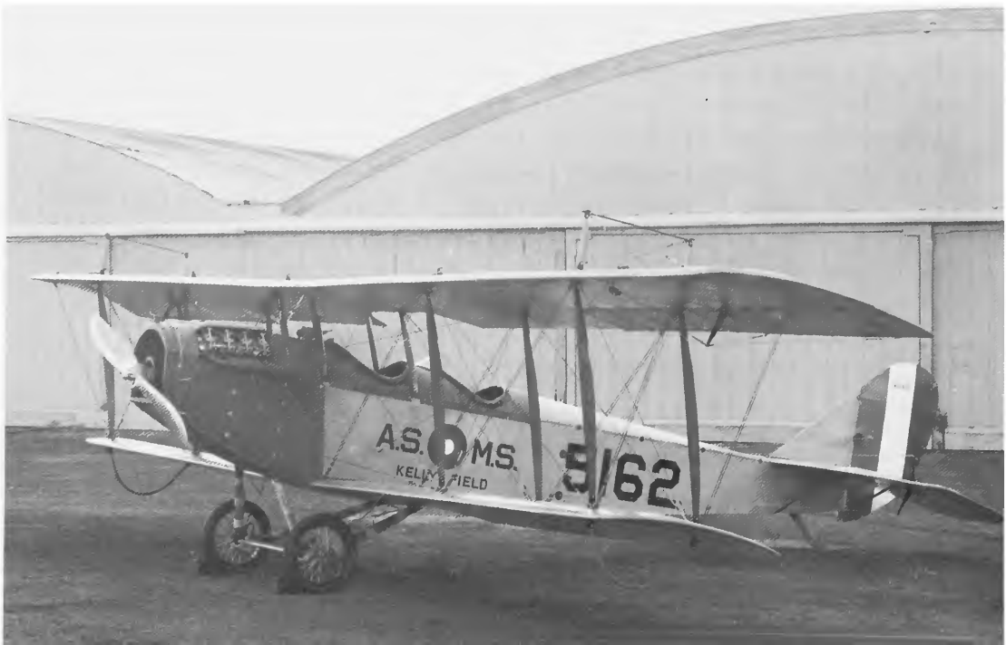
Figure 23.—Curtiss JN-4 Jenny airplane with OX-5 engine, 1915. (Photo courtesy Harrah's Automotive Museum, Reno, Nevada)
