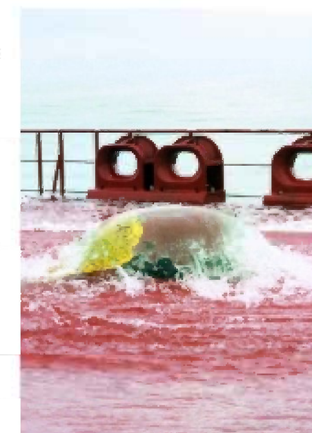
Ballast water exchange on Berge Nord is performed using the "300% flow-through method".
