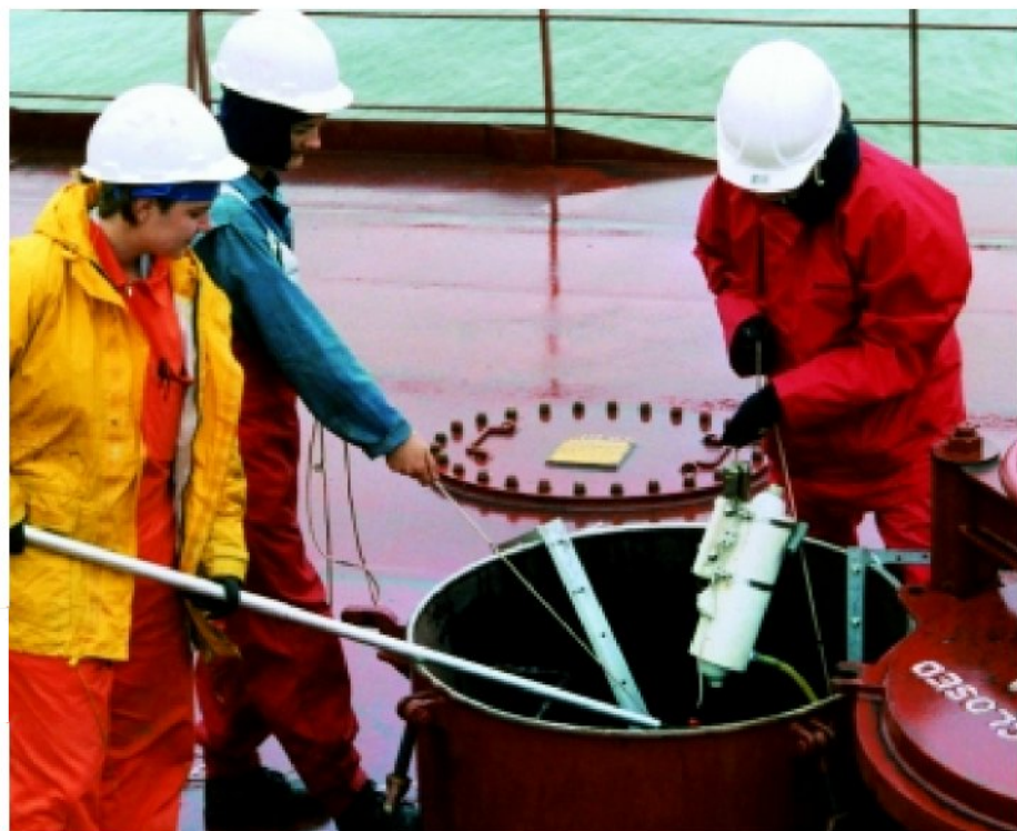
The scientists are sampling the ballast water of the Berge Nord.
