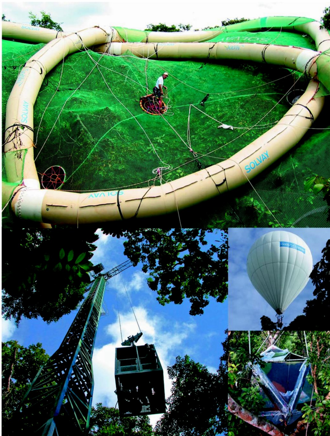
Plate 2 — Canopy access devices, clockwise: SolVin-Bretzel canopy raft, canopy bubble, Ikos tree house and canopy crane. Photos: S. Bechet, R. Le Guen, JO, ML.
