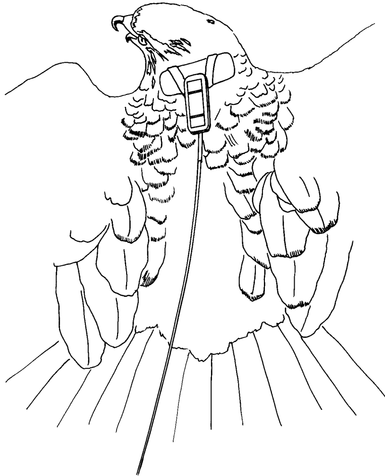
FIGURE 1. Solar-powered transmitter and feather shield in place on back of nestling Snail Kite.
