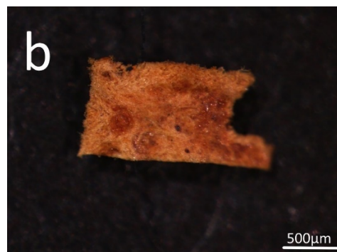
Figure 6. Microscope photos of gold lamellae (object no. 6, samples from ear) showing the presence of follicles (a) on the grain side and; (b) fibrous structure on the underside ©Conservation Office
