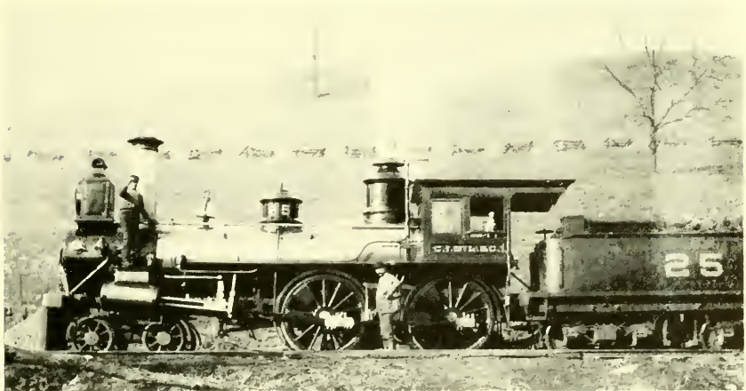
Figure 18.—ENGINE NO. 25, BUILT IN 1864 BY MOORE & RICHARDSON for the Indianapolis and Cincinnati Railroad, later the Cleveland, Cincinnati, Chicago, and St. Louis Railroad. Shown as rebuilt in 1882 with a new boiler.
