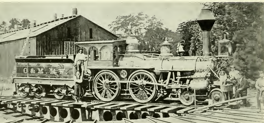
Figure 47.—A NILES-BUILT OHIO AND MISSISSIPPI LOCOMOTIVE, probably constructed in 1854. Shown here as rebuilt for standard gauge in about 1871. Original number and scene unknown.
