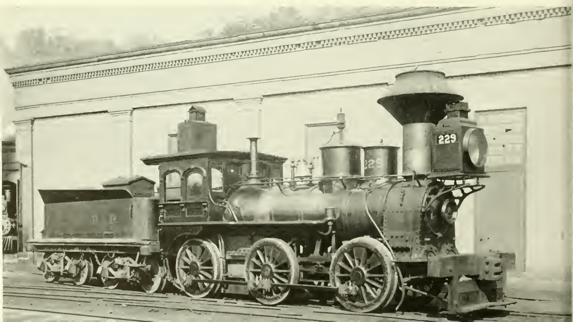
Figure 16.—THE "COLUMBUS," A 6-WHEEL SWITCHER rebuilt in 1865 at the Pendleton Shops of the Little Miami Railroad. Probably was a Moore & Richardson 4-6-0 of the 1850's.
